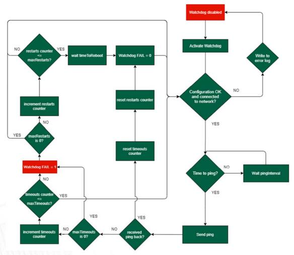
Figure 36 - Watchdogs flow diagram
