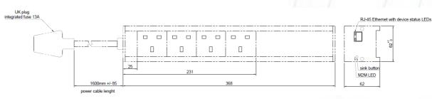
Figure 6 - PoweBOX 4KG front and side view [mm]
