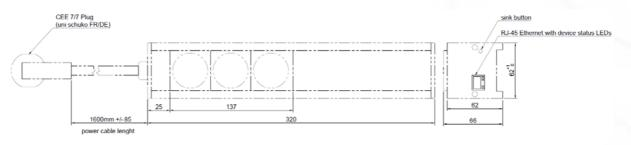
Figure 2 - PoweBOX 3Px front and side view [mm]
