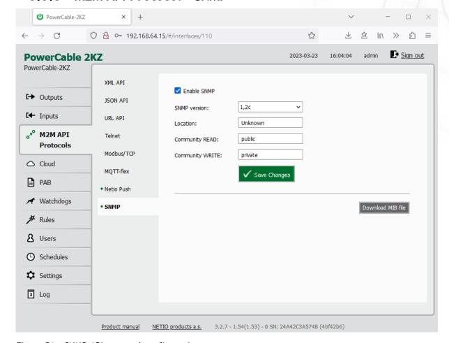
Figure 51 - SNMP API protocol configuration
