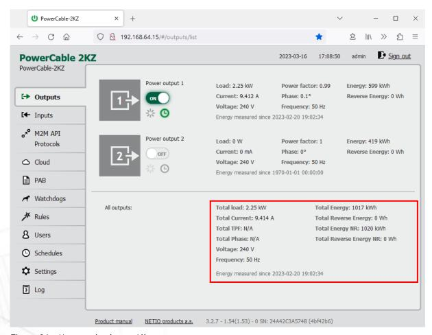
Figure 36 - Measured values - All outputs
