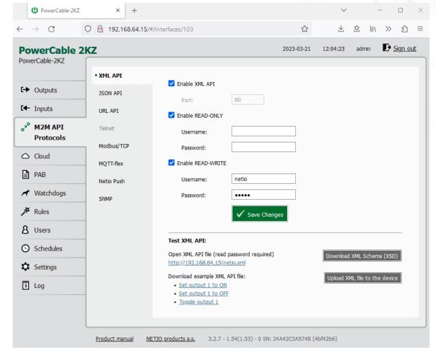
Figure 42 - XML API protocol configuration
