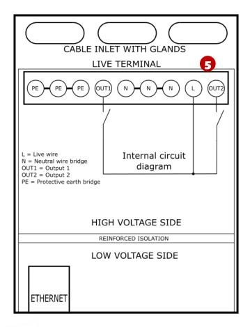
Figure 14 - PoweCable 2PZ top view
