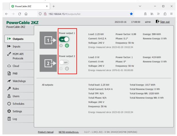
Figure 34 - Controlling the output
