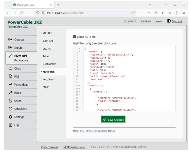
Figure 49 - MQTT-flex protocol configuration
