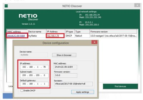
Figure 30 - Discovering network parameters using NETIO Discover
