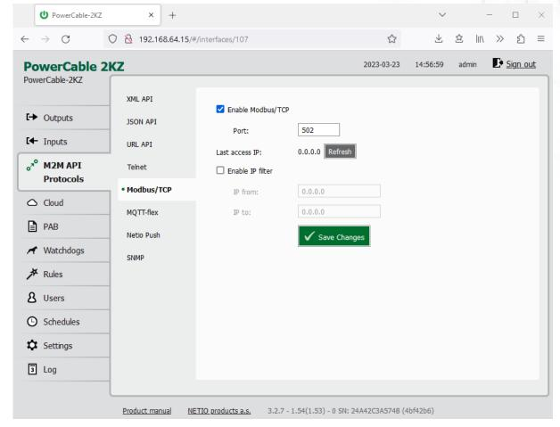
Figure 48 - Modbus/TCP protocol configuration
