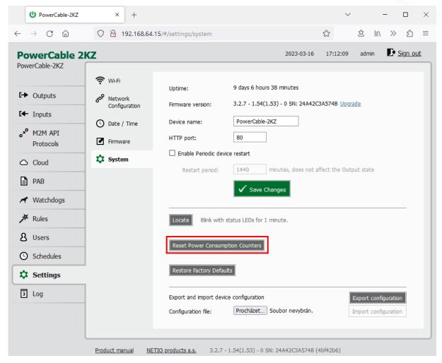
Figure 37 - Resetting the consumption counters
