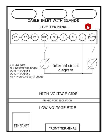
Figure 16 - PoweCable 2PZ top view
