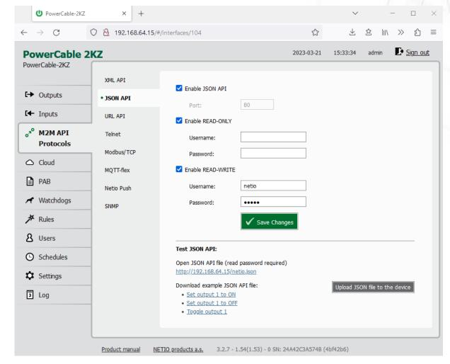
Figure 44 - JSON API protocol configuration
