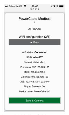
Figure 27 - Configured Wi-Fi parameters
