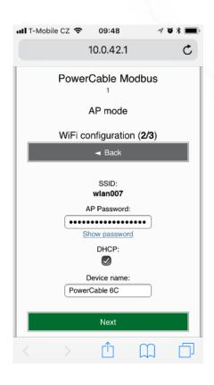
Figure 25 - Connecting to Wi-Fi in AP mode
