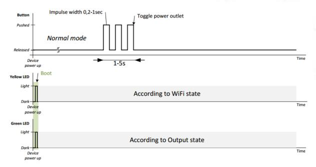
Figure 33 - LED indication for manual output control
