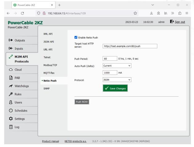
Figure 50 -Netio Push protocol configuration
