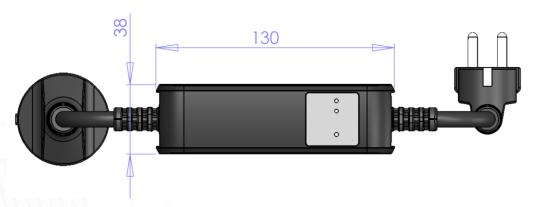
Figure 13 - PoweCable xxx 101x top view
