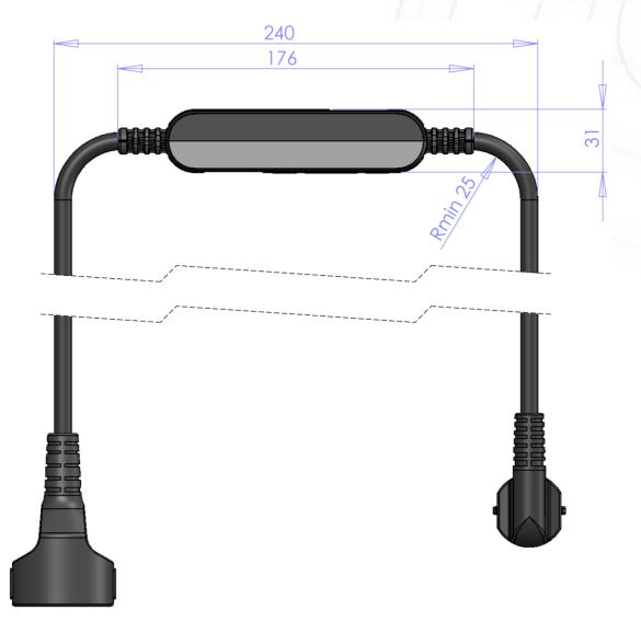
Figure 12 - PoweCable xxx 101x side view
