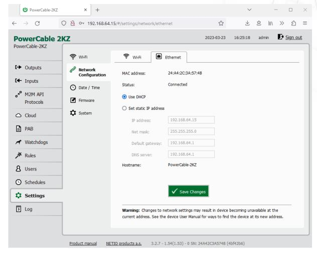
Figure 63 - Network configuration - Ethernet
