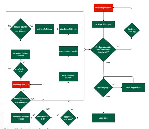
Figure 55 - Watchdogs flow diagram
