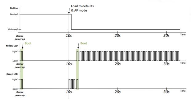
Figure 32 - LED indication when restoring factory defaults
